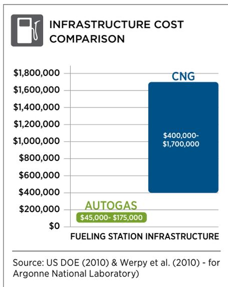
A small, fast-fill CNG station costs approximately \$400,000, according to a 2010 Department of Energy study on the feasibility of natural gas vehicles. Fast-fill dispensers are the preferred option for most fleet and public fueling stations, as they provide similar fill times to gasoline pumps.
